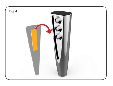
Remove the orange outer protection film from the double sided tape.
